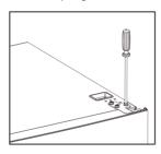
3.Remove the pin with a screwdriver and filp the hinge bracket. Then refit the pin to hinge bracket
