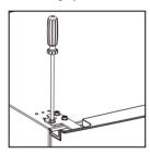
16.Connect harnesses from door and cabinet. Then replace top hinge cover. Before screw the cover, connect terminals of door switch.
