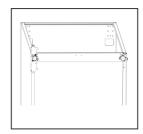
12.Remove aid-closers from bottom of upper and lower doors, then take new aid-closers from accessary bag and install them to left side.
