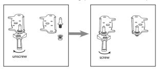
11.Refit the bracket fitting the bottom hinge pin. Replace both adjustable feet.
