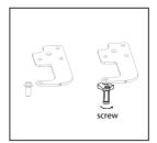
4. Move door switch from right hinge cover to left hinge cover in accessary bag.
