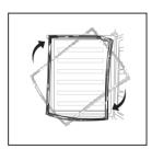
14. Install the lower door, adjust and fix the middle hinge onto the cabinet.
